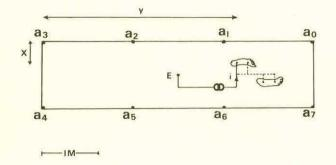
Fig. 1. Schematic diagram of walkway with position of two feet and electrodes. The current flows from one of the four footsole electrodes to electrode E, in the centre of the mat. Potentials are measured relative to electrode a at positions a to a 7.
