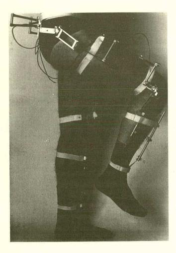
Figure 2. Side view of self-aligning goniometers for simultaneous flexion angle measurements of both hips and both knees, showing the method of attachment to thigh and shank, and the adjustable supports for potentiometers and linkage guides.
