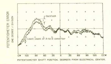
Figure 5. Typical calibration curve for a precision potentiometer with conductive plastic resistance element. The vertical scale represents deviation of the potentiometer output from perfect independent linearity. Errors result from nonuniformity in the resistance element, backlash in the wiper, and limited resolution of the analog-to-digital converter that is used to measure potentiometer output.
