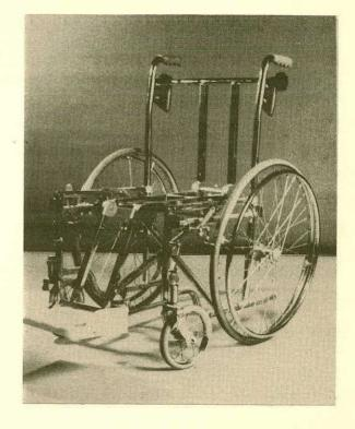
Photo 7 Adjustable insert frame on 18" E & J wheelchair.
