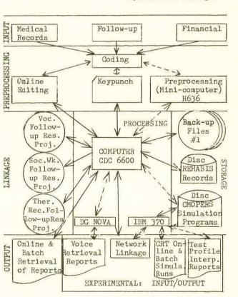
Figure 2. Schematic representation of the REHABIS data linkage
