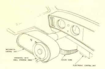
Figure 1. Perspective View of Servo-Mechanical Steering Control Device •
