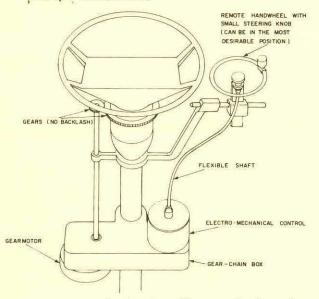
Figure 8. Handwheel with small steering knob can be in the most desirable position (with conventional steering wheel on).
