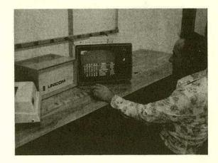
Figure 1. UNICOM system, with printer, processor and video display.
