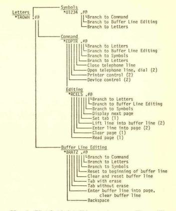
Fig. 3 Flowchart detailing system operation. (1) and (2) indicate number of digits needed in a numerical modifier to completely specify the corresponding command.
