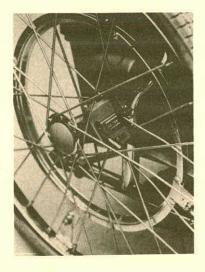
FIGURE 1. Wheelchair odometer, installed on an electric-powered wheelchair.
