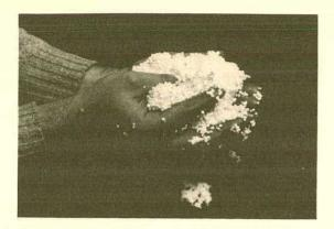
Figure 2. Photograph of a handful of the fluidized-bead mixture.
