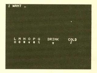
Figure 4b. Same as Figure 3a, except key "\*"has been pressed. Pressing " $\psi$ " will cause the word "DRINK" to be transferred to the message space starting at the underscore cursor location.
