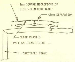
Figure 4. Optics for code display integral with gaze target presentation. The spacing between a viewing lens and its code transparency must be accurately set to permit clear vision with a comfortable state of focus of the eye.
