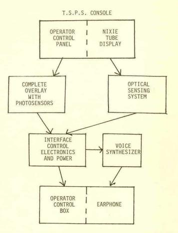
Figure A-1 Prototype T.S.P.S. Interface Equipment - Schematic
