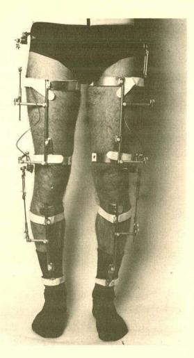
Figure 3. Front view of the self-aligning goniometers showing close fit of linkages to the body.
