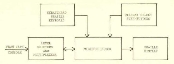
Figure 2. Block diagram of TSPS braille display
