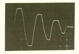
Figure 5. Generating the sequence of levels: +3,-3,+2,-2,+1,-1,0, by volume control. Scan rate: 2 s/cm
