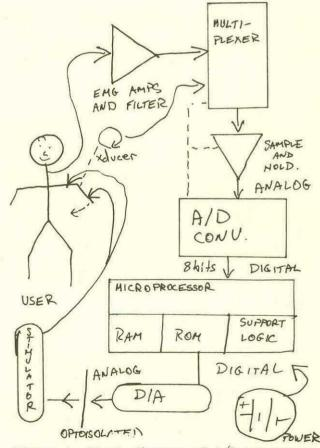
Figure 1: Block diagram of A/D, processor, and D/A.
