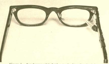
Figure 1. Eyeglasses with Optics to Monitor Eye Position
