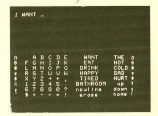
Figure 4a. UNICOM screen while operating in a 9-key encoding mode (8 select and a clear key). Each key selects a row if used now. The symbols on the sides of the matrix are marked on their respective keys.
