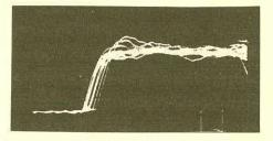
Figure 2b. Maintaining a constant flow by exhalation (10 attempts). Scan rate: 0.2 s/cm
