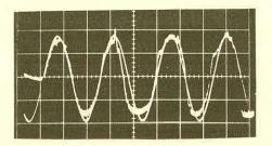
Figure 4a. Attempting to track by airflow a 2 Hz sinewave. Scan rate: 0.2 s/cm
