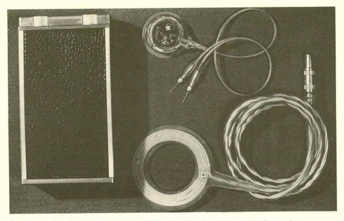
Figure 2. Typical stimulation system showing the power supply/transmitter unit , implanted receiver/stimulator and coupling antenna. These particular units are made by Avery Laboratories.
