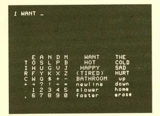
Figure 3b. Same as Figure 3a, except 4th row has been selected by switch closure. The cursor, a set of parentheses, is moving across the matrix. If the switch were closed at this time the word "TIRED" would be transferred to the message space starting at the location where the underscore is positioned.
