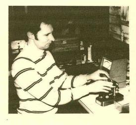
Figure A-2 Machinist Taking Precision Measurements With Adapted Dial Gauge
