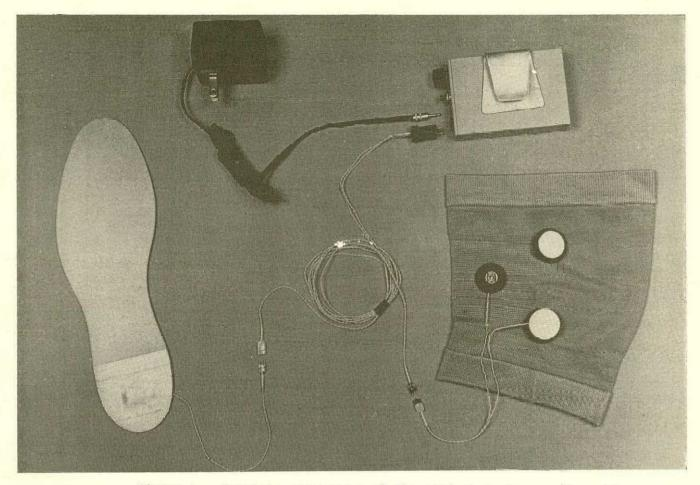
Figure 1. Complete components of the patient system: unit, cable assembly, battery charger and innersole.
