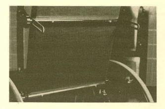
Photo 8 Simple insert hardware. Top, crosstube and pivotting slotted brackets. Bottom, crosstube and open clips.
