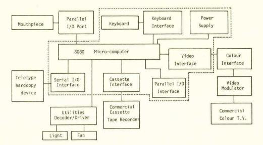
Fig. 1 Block Diagram of Environmental Controller
