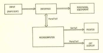
Fig. 1 Block diagram of microcomputer-based control and communication system.
