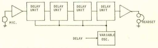
Figure 1: Block diagram of the solid-state DAF unit.
