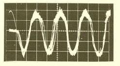
Figure 4b. Five attempts of the type shown in Figure 4a. Scan rate: 0.2 s/cm
