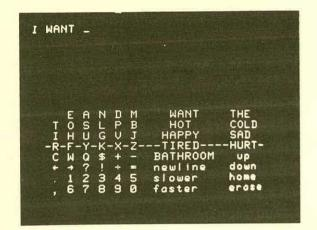
Figure 3a. UNICOM screen while operating as a row-column scanning mode, i.e. TIC style. The message space is the top 7 lines, the input matrix the bottom 8 lines. The horizontal row of dashes is the row cursor.
