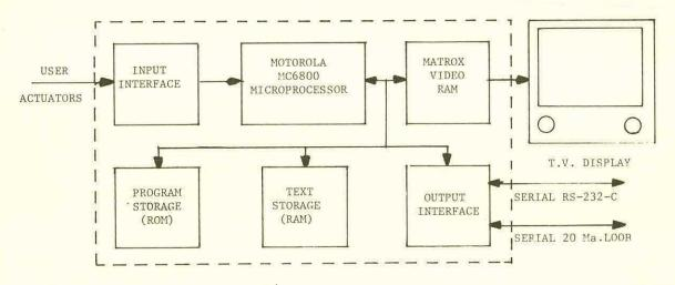
Figure 2. UNICOM Block Diagram.
