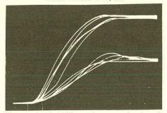
Figure 6. Settling at a constant volume level; 5 attempts each. Scan rate:.2 s/cm
