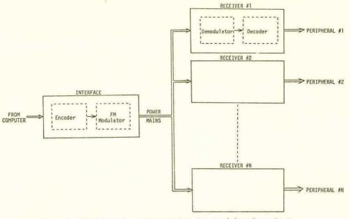
Fig. 4 Vistributed controx system for peripheral controx.
